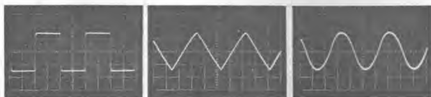
Figure 4-10. Oscillograms showing the operation of the integrating circuits in the vibration meter. In (A) a square wave is shown as transmitted by the amplifier when set for acceleration measurements. (B) shows the wave after one stage of electrical integration for velocity measurements, and (C) shows the result of two stages of integration as used for displacement measurements.
