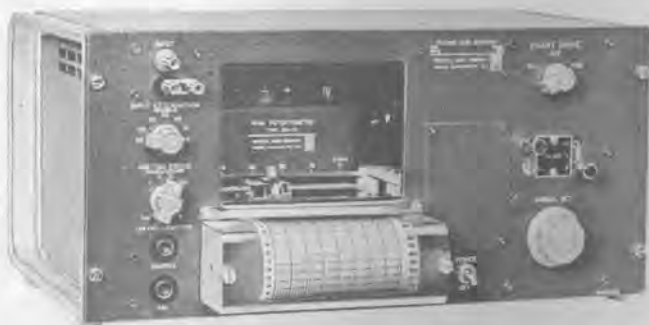
Figure 4-21. The Type 1521-B Graphic Level Recorder.
