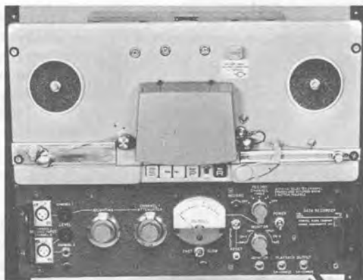
Figure 4-27. The 1525-A Data Recorder shown with Tape loop for analysis of short-duration signals.
