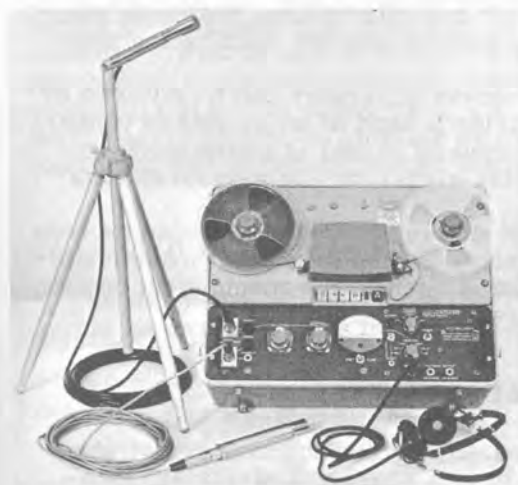
Figure 4-28. The 1525-A Data Recorder with Pre-amplifiers and micro-phones at both input channels and headphones at its "monitor" jack.
