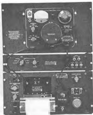
Figure 4-24. The Types 1564 Sound and Vibration Analyzer, 1521-B Graphic Level Recorder, and 1564-P1 Dial Drive assembled for automatic 1/3-octave testing.
