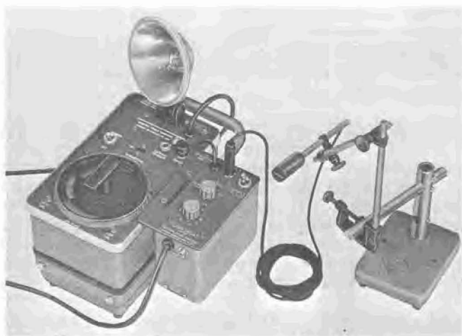
Figure 7-12. An electronic stroboscope arranged for triggering from a photoelectric pickoff with an adjustable delay. These instruments were used to obtain the photographs of the cam and follower.
